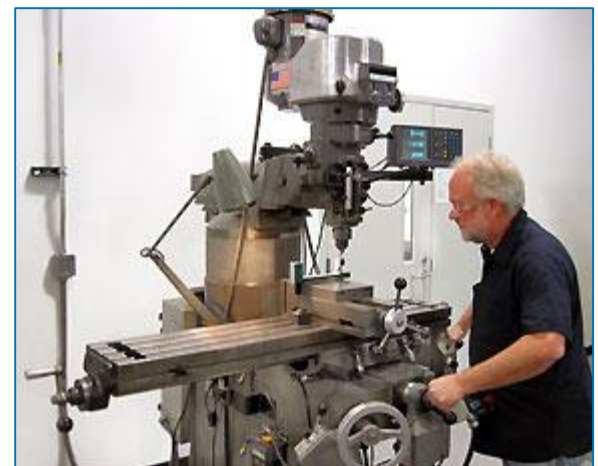
Vertical Milling Machine produces prototypes, tooling and fixtures to precise dimensions.
