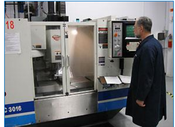
Computerized Numeric Control (CNC) Mill creates metal and plastic prototype parts from models or prints.
