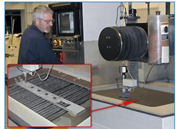
Water Jet Cutter offers low cost, precision cutting of complex shapes.
