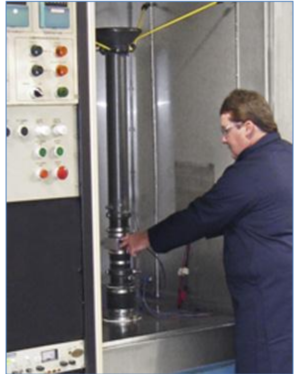
Temperature and Humidity Compensated Air Flow Test Stand at Delphi's Customer Technology Center Michigan Technology Center Michigan
