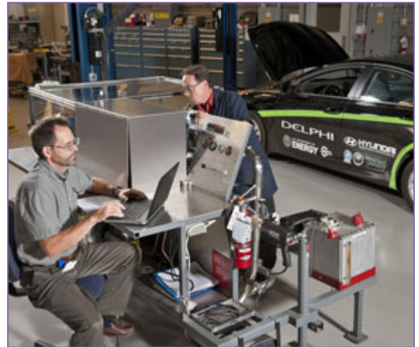
Advanced powertrain controls development using a test cart is underway at the Delphi CTCM Vehicle Test Lab.
