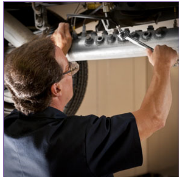
Installing exhaust sensors for development testing in the Delphi CTCM Vehicle Test Lab.
