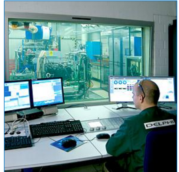
Engine Dynamometer Control Room at Delphi Customer Technology Centre Luxembourg
