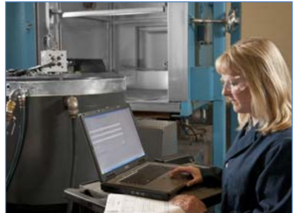
Environmental Chamber/Shaker Table in the Vibration Laboratory at Delphi's Customer Technology Center Michigan
