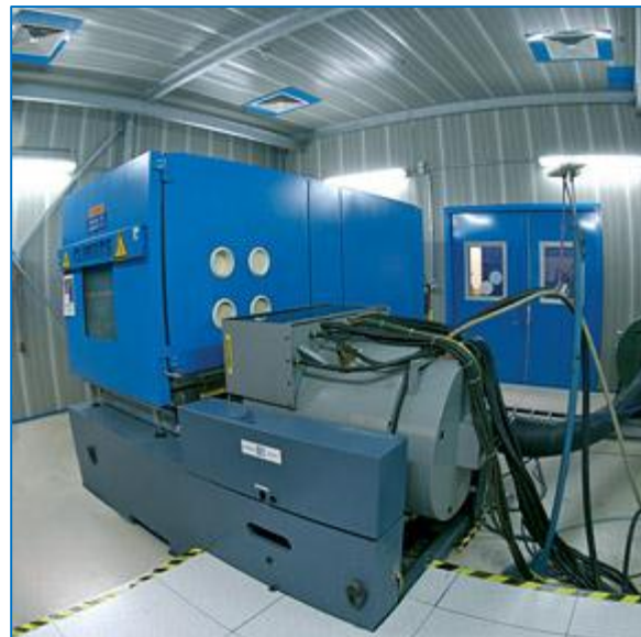
Electrodynamic Shaker at Delphi Customer Technology Centre Luxembourg
