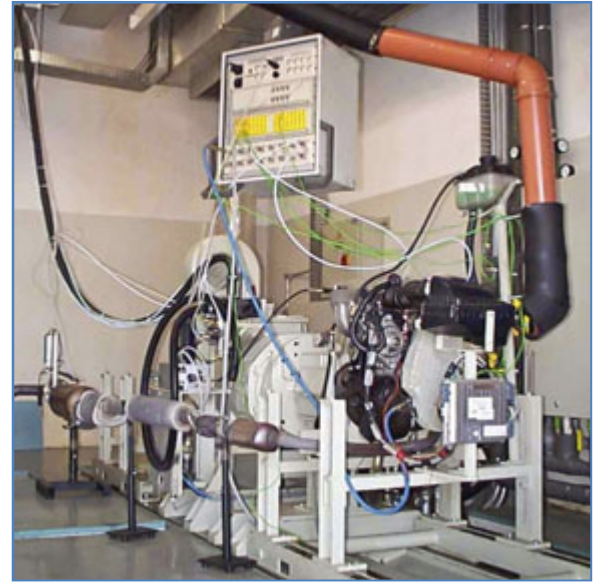
Engine Dyno Test Cell in the TCP Engine Dynamometer Laboratory.
