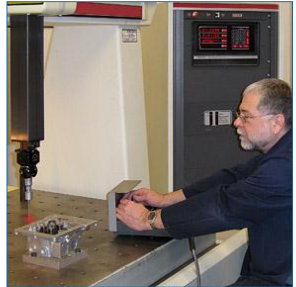
Operator at Coordinate Measuring Machine in the Dimensional Measurement Services Laboratory at the Delphi Customer Technology Center Michigan
