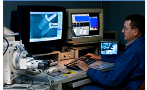
Scanning electron microscopy (SEM) services include inspection of semi-solids and non-conductors with magnifications up to 300,000 times.
