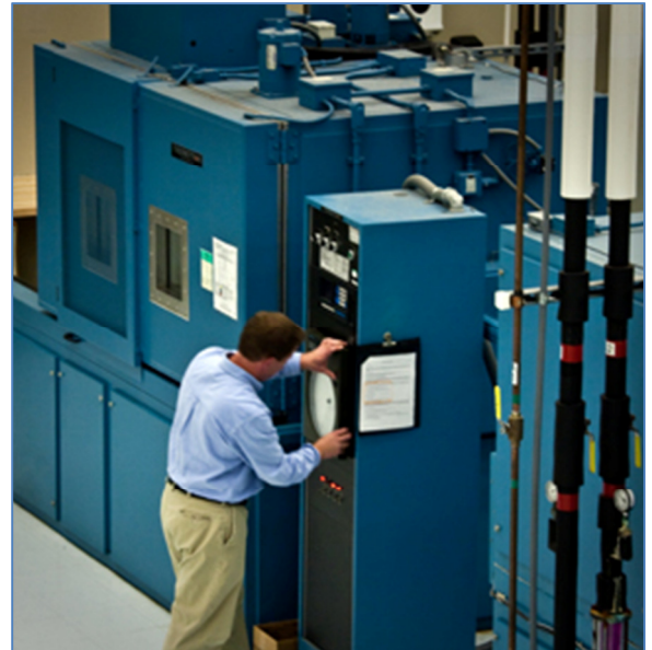
Environmental chambers enable testing in many conditions, including dust, salt, extreme temperatures, and more.
