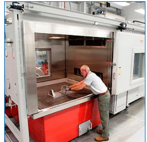
Combined Environment System: Vibration (15,000 Lbf) / Temperature / Humidity
