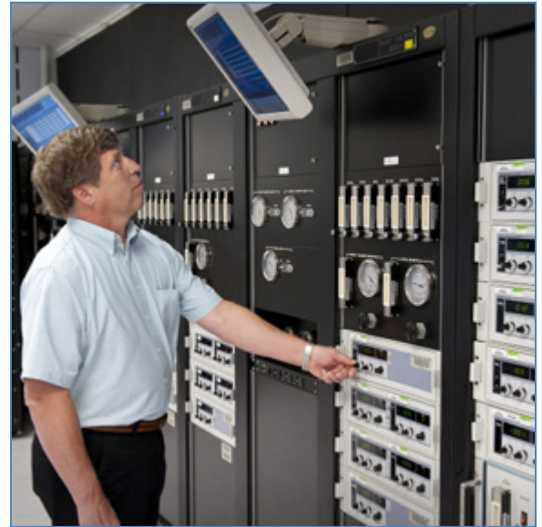
An engineer makes adjustments on a Tailpipe Emissions Bench in the Vehicle Emissions Testing Laboratory at the Delphi Customer Technology Center Michigan.
