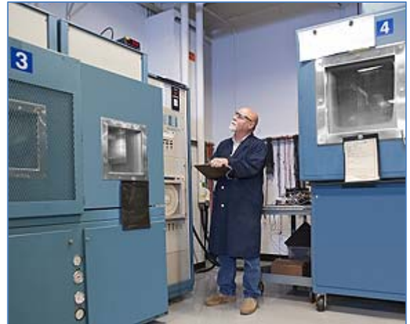
The Thermal Shock Chamber at the Delphi CTCM has a maximum operating temperature up to 250°C.
