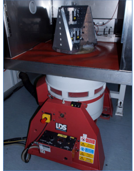
Vibration / Shock Testing
