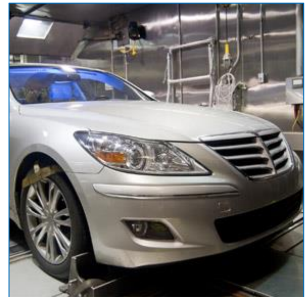
The Environmental Capable Chamber in the Vehicle Emissions Testing Laboratory at Delphi's Technical Center Rochester
