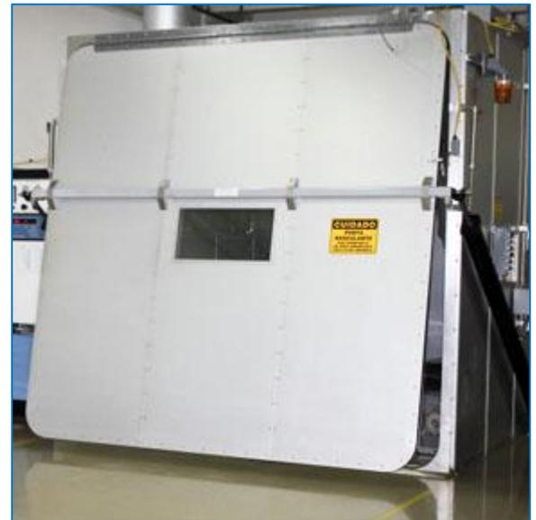
**Climatic Chamber at the Delphi TCP VE Lab.**
