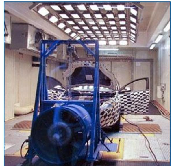
**Sealed Housing for Evaporative Emissions Determination (SHED) chamber at the TCP VE Lab.**
