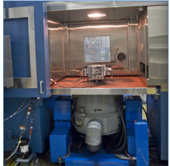
Typical set-up for the Vibration Laboratory at Delphi's Technical Center Rochester
